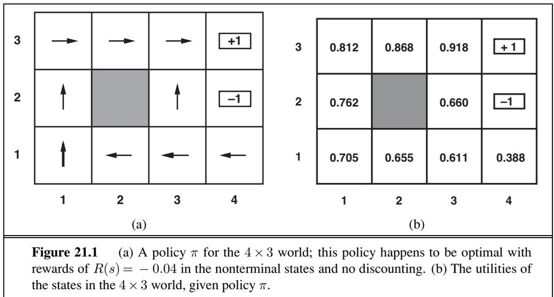
**Figure 21.1** (a) A policy  $\pi$  for the  $4 \times 3$  world; this policy happens to be optimal with rewards of  $R(s) = -0.04$  in the nonterminal states and no discounting. (b) The utilities of the states in the  $4 \times 3$  world, given policy  $\pi$ .
