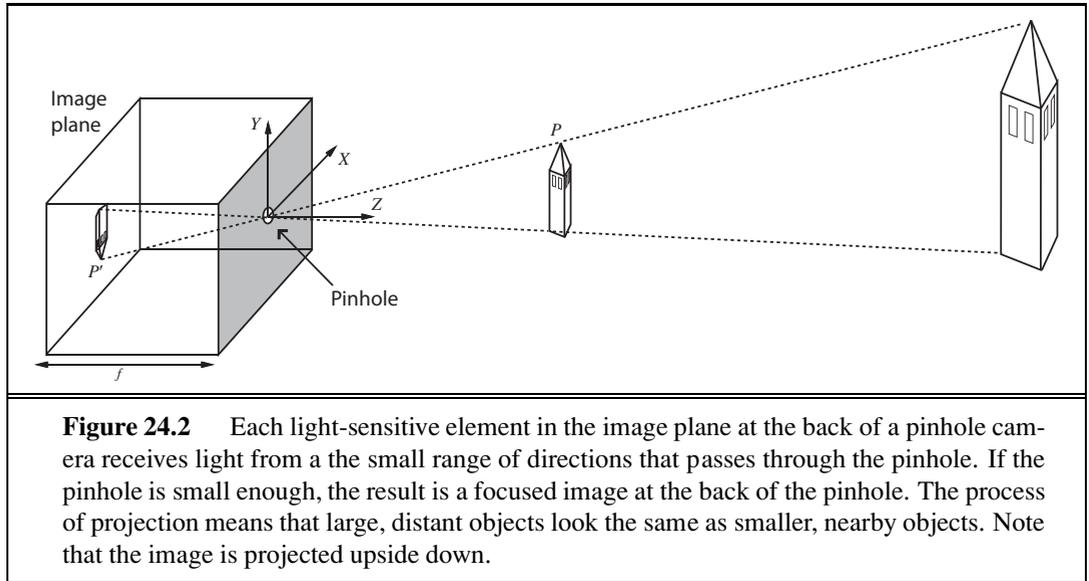
**Figure 24.2** Each light-sensitive element in the image plane at the back of a pinhole camera receives light from a the small range of directions that passes through the pinhole. If the pinhole is small enough, the result is a focused image at the back of the pinhole. The process of projection means that large, distant objects look the same as smaller, nearby objects. Note that the image is projected upside down.
