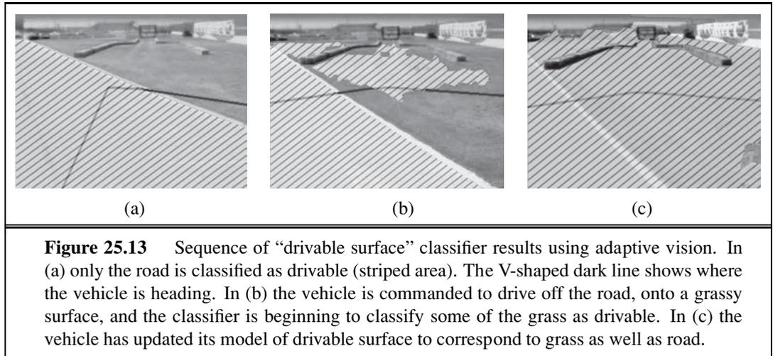
**Figure 25.13** Sequence of “drivable surface” classifier results using adaptive vision. In (a) only the road is classified as drivable (striped area). The V-shaped dark line shows where the vehicle is heading. In (b) the vehicle is commanded to drive off the road, onto a grassy surface, and the classifier is beginning to classify some of the grass as drivable. In (c) the vehicle has updated its model of drivable surface to correspond to grass as well as road.
