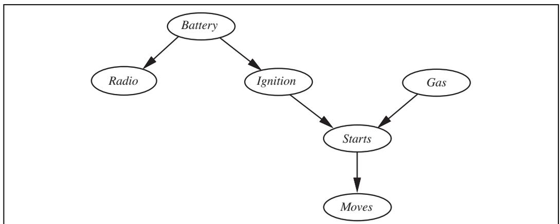
**Figure 14.21** A Bayesian network describing some features of a car's electrical system and engine. Each variable is Boolean, and the *true* value indicates that the corresponding aspect of the vehicle is in working order.
