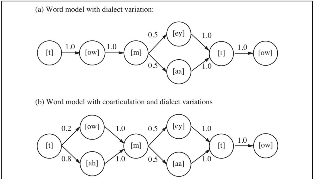
**Figure 23.17** Two pronunciation models of the word “tomato.” Each model is shown as a transition diagram with states as circles and arrows showing allowed transitions with their associated probabilities. (a) A model allowing for dialect differences. The 0.5 numbers are estimates based on the two authors’ preferred pronunciations. (b) A model with a coarticulation effect on the first vowel, allowing either the [ow] or the [ah] phone.
