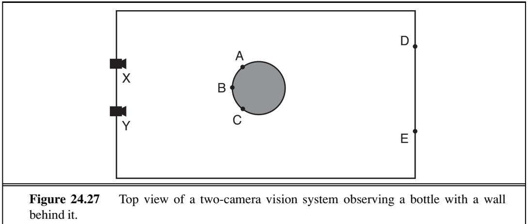
**Figure 24.27** Top view of a two-camera vision system observing a bottle with a wall behind it.
