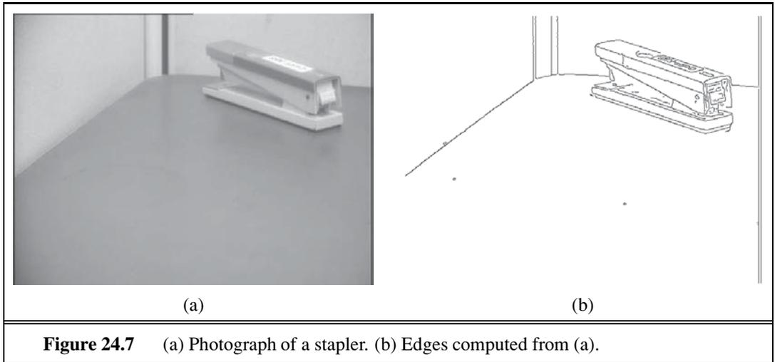
**Figure 24.7** (a) Photograph of a stapler. (b) Edges computed from (a).
